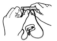
5. Pull cords through into glider channel and clear of cutting point.
