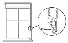
The P-Clip chain tensioner must be fitted at the maximum distance possible from the control mechanism to prevent the chain loop from becoming slack. With the chain inside the P-Clip, position it on the wall making sure the chain is taut yet still able to move freely. Mark the screw hole(s) with a pencil and attach it to the wall with the fixings provided. Please note it is a requirement in accordance with BS EN 13120 to install the P-Clip and the installer is liable to ensure child safety.
